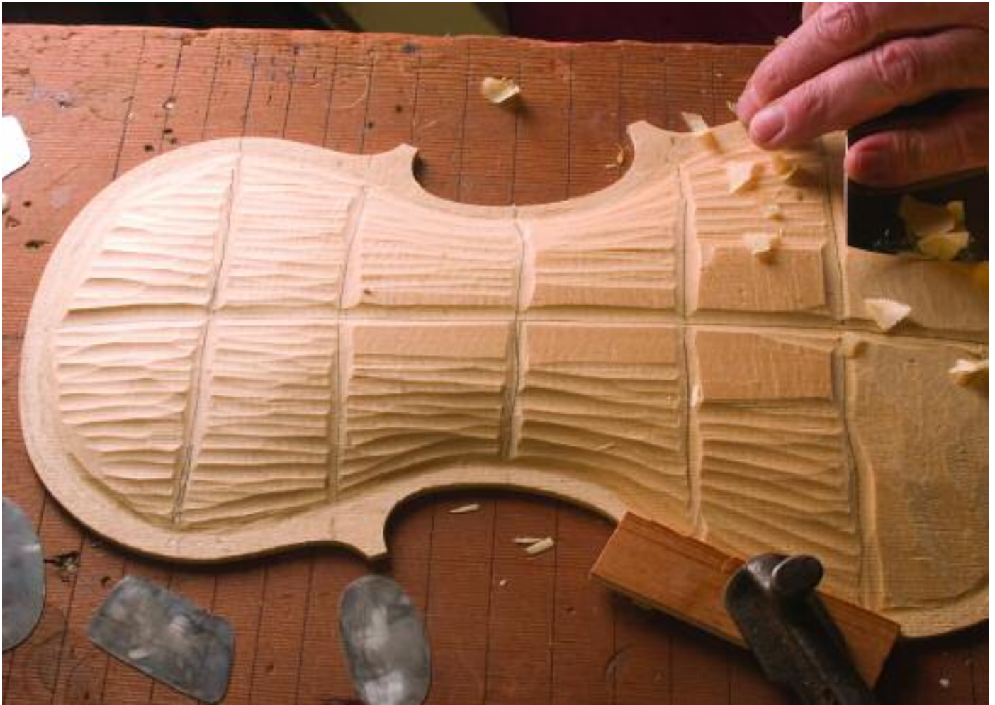
David Chrapkiewicz uses a gouge to carve the top of a violin from two joined pieces of German spruce.
