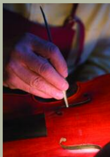
The sound holes are cut with a small, fine saw and finished with a razor sharp, fine-pointed knife.
